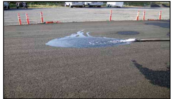
Permeable asphalt absorbs rain water at the rate of 100 inches per hour.
